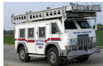
Nyala RG-12 used by London police, with MARS ladder system used for entering planes or buildings.
